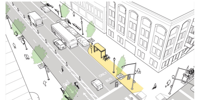
A bus bulb station
