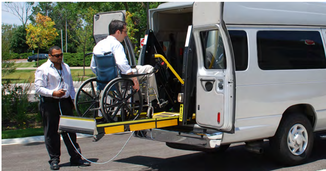
A wheelchair lift in operation.
