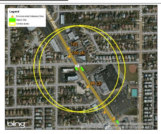
The northbound Ballard Road station is planned to be constructed in the grassy terrace between the curb and sidewalk, adjacent to a vacant lot. The southbound Ballard Road station is planned to be constructed at the same location as the existing southbound Pace bus stop, adjacent to the PNC Bank property.
